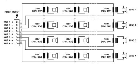
diagram 3 Connection of 100 V (70 V or 50 V) loudspeaker systems
